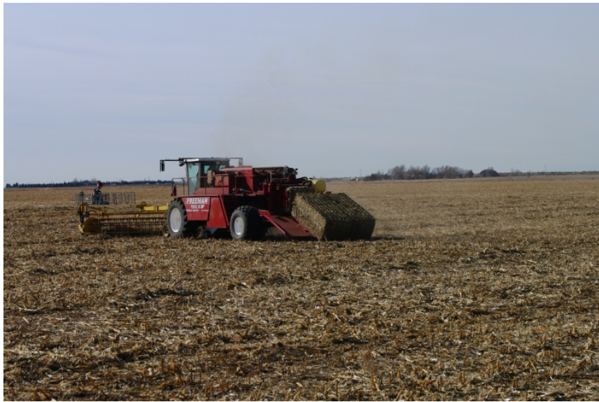
The self-propelled baler collects and packages bales of feedstock on-site that can be immediately loaded and sent to a biorefinery for use. | Photo courtesy of Antares Group.
