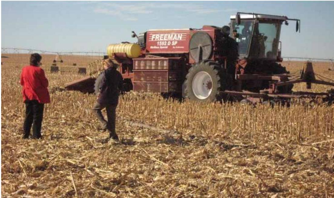
FDC Enterprise’s Feedstock Logistics award has developed a single pass harvester, which is shown gathering corn stover and feeding it into the baler. Thanks to strategic modifications to the harvester, tightly packed, large square bales emerge from the rear of the baler and are gently lowered to the ground in pairs while the baler continues its job. | Department of Energy Photo.
