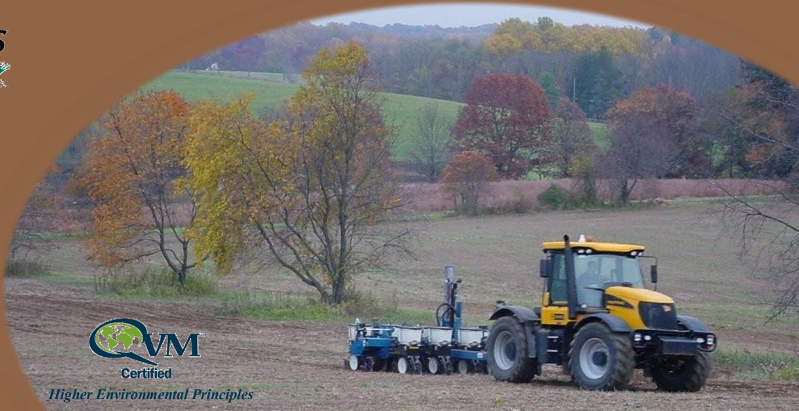
Custom built planters; modified to plant and spray native grasses
